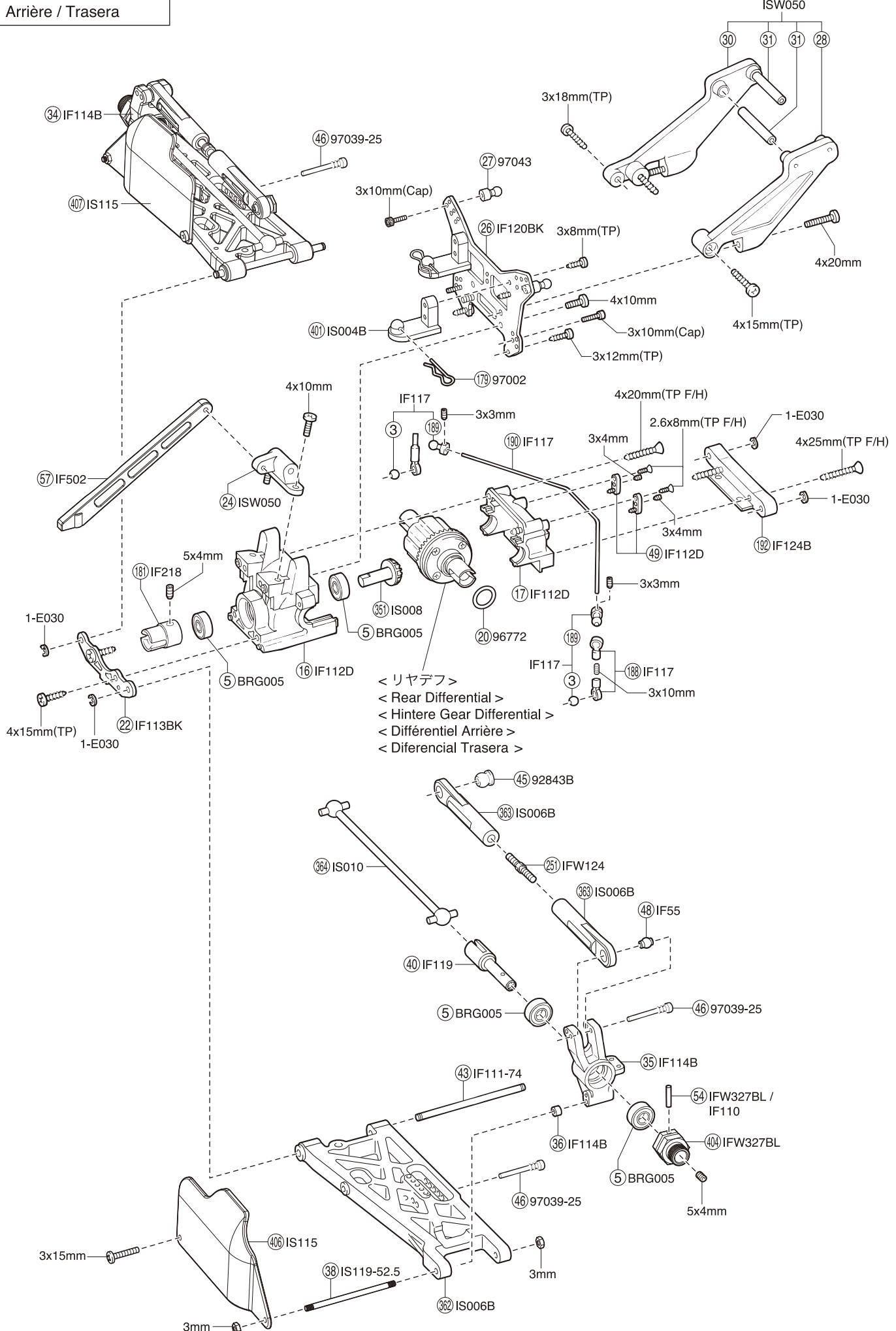
デフギヤ / Differential / Gear Differential
